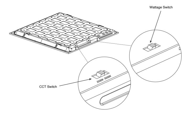
The end users may adjust the color temperature and lumen output respectively by the two DIP switch buttons integrated into the driver. Each DIP switch is accommodated with 3 options (left, middle and right), corresponding to 3 color temperatures and 3 powers respectively, which can perform the desired color temperature and lumen output combination.
