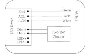
Follow wire connection instructions. When using the 0-10V dimming controller Run wires from controller through a different knockout than the AC input wire. Don't forget to return the electrical enclosure cover and tighten the screws.
