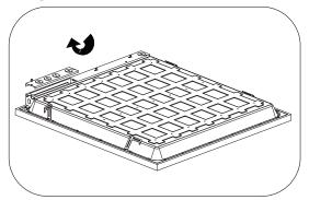
Remove electrical enclosure cover. Carefully remove knockout for AC line input wires and 0-10V control line. Install listed electrical fittings in the knockout holes for wire protection if needed.
