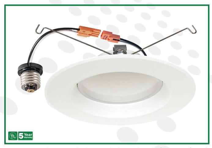
Our JET LED Down Light is economical and is equipped with a smooth trim that fits most manufacturer's 5" and 6" recessed can-style housings. It utilizes adjustable torsion springs, can be dimmed down to 10%, and maintains 70% light output after 35,000 hours of use. This makes it perfect for applications such as multi-family residences, retail shops and offices. An E26 adapter is included.
