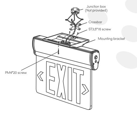
5. Now connect the wires. If you're using 120V AC, connect the black and white wires to the building wires. If you're using 277V AC, connect the red and white wires to the building wires.
