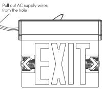
5. Now connect the wires. If you're using 120V AC, connect the black and white wires to the building wires. If you're using 277V AC, connect the red and white wires to the building wires. 6. Attach the mounting bracket to the crossbar with the PM4\*20 screws. 7. If the chevrons are needed, PLEASE keep them and tear off the instruction stickers on the panel. If not needed, tear off all the stickers on the panel.
