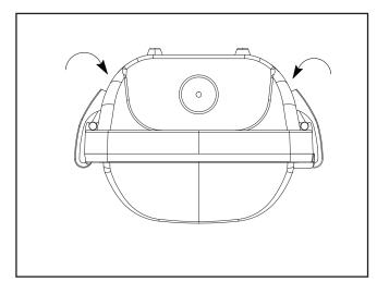
7. Reattach LED tray and lens to fixture by reversing step 4.
