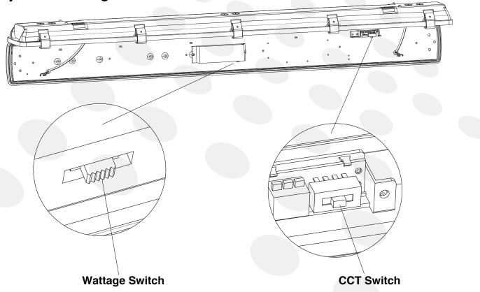
The end users may adjust the color temperature and lumen output respectively by the two DIP switch. Each DIP switch is accommodated with 3 options (left, middle and right ),corresponding to 3 color temperatures and 3 powers respectively, which can perform the desired color temperature and lumen output combination.
