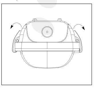
5.Without touching LED boards,detach LED tray and lens from fixture.
