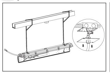
9.Secure lens to housing with lens latches.
