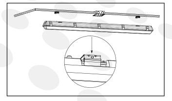
4. Without touching LED boards, detach LED tray and lens from fixture.
