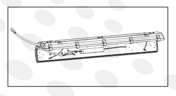
8.Reattach LED tray and lens to fixture by reversing step 5.
