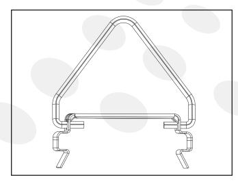
2. Secure mounting clips to housing recesses by firmly pressing them into place until both sides of the clip are secured. Hang fixture from customer supplied chain using V-brackets.
