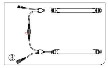
3. Tighten the nut of the connector.
