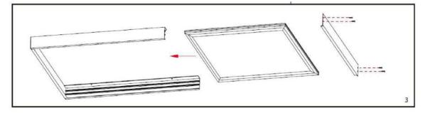
4. Fix the frame by putting back the dismantled part.
