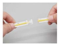
Insert each end of led strips into the end of the connection terminal respectively, make sure the metal clip is in same side as the metal solder pad of led strip.
