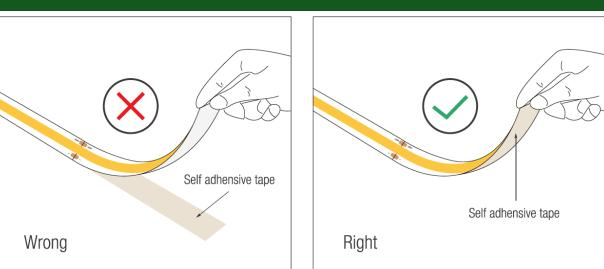
If the led strip needs to be torn upwards, please make sure that the self adhesive tape is torn with the led strip, else the led strip would be damaged.
