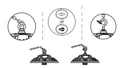
2. First fix the hook on the lamp (rotate clockwise) then connect the hook with the lock ring
