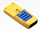
Check the direction of the batteries and insert them one at a time.
