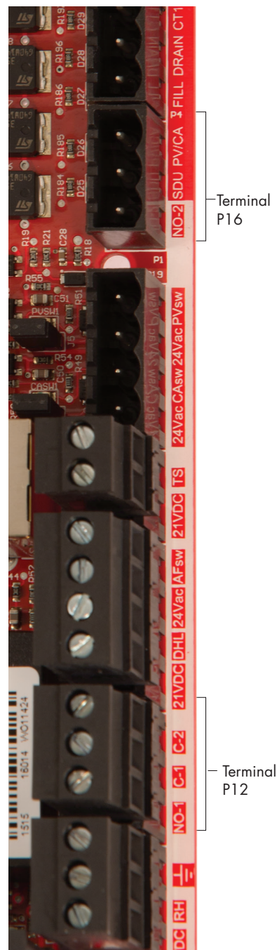
FIGURE 19-1: TERMINAL P12 AND P16
