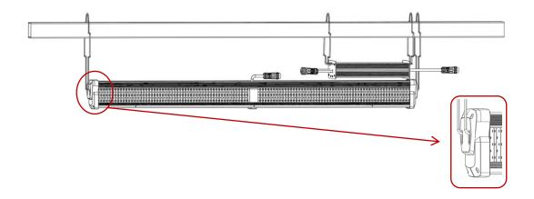
2. Connect the DC power cord between light fixture and driver.
