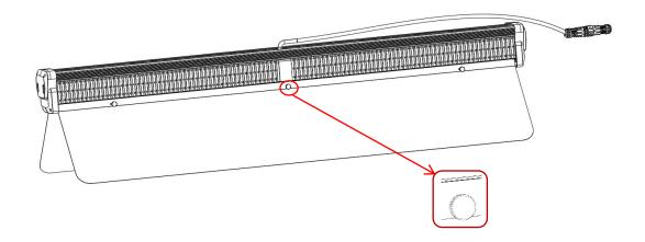
4. If using 0-10V dimming control, then connect dimming port on the driver to another light fixture or dimming controller by linking cords.
