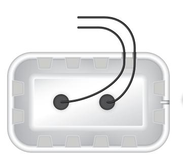
Connect the Air Pump Tubing to the end of the Air Stones. Arrange the tubing into the channels located on rim of the Reservoir.
