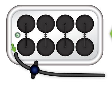
Run the short end of the preassembled Ball Valve and Drain Tube through the hole in the lid and connect it to the tubing on the underside of the lid.
