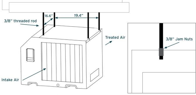
Parts Needed: 4 pieces - 3/8" threaded rod (not included) 4 pieces - 3/8" threaded jam nuts (not included)
