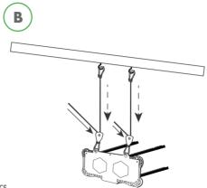
Lift the LED and attach the carabiners to pre-installed hooks from ceiling or mounting beam. The Ratchets should be installed closest to the LED (and not the ceiling).
