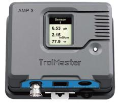
Connect the AMP-3 Sensor to the NFS-2 main controller using an RJ12 cable via "System" terminal ; the pH Sensor via the BNC terminal; EC/TEMP terminal via Mini DIN terminal. Once connected, pH level, EC level and water temperature will be displayed on both the AMP-3 LCD screen and the Aqua-X Pro master controller screen.
