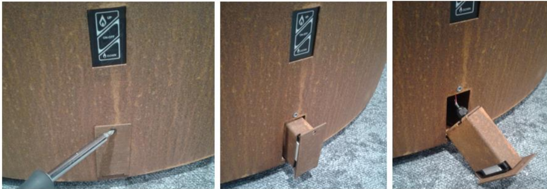
Photo 6: Removing of the battery container
