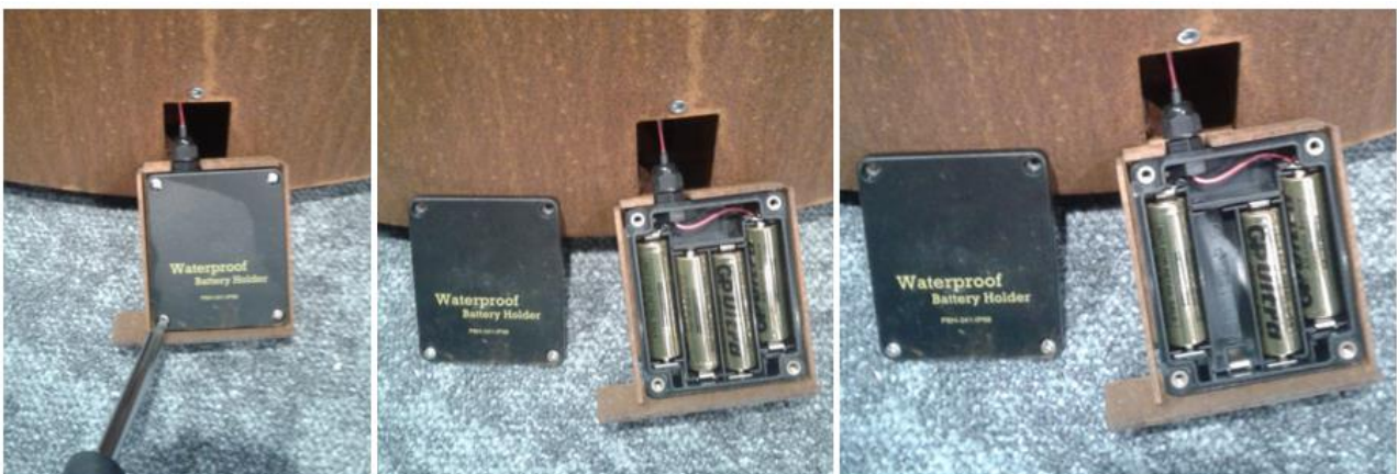
Photo 9: Replacing the batteries in the container
