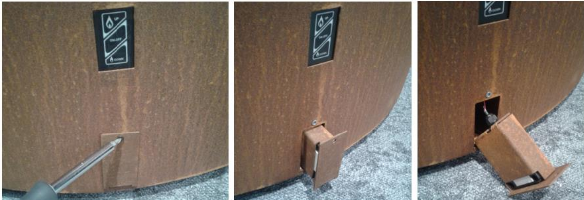
Photo 6: Removing of the battery container
