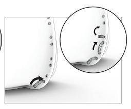
3. Thread the rope through the next hole above and pull towards the internal of the planter. Thread the rope in alternating in-out pattern as illustrated.
