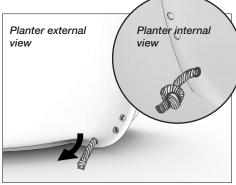
2. Pull the unknotted end of the rope all the way through the hole until the knot hits the end as shown.
