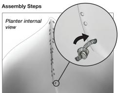
Locate the last hole on one side of the planter. Tie a simple knot on the end of one of the ropes and thread unknotted end through hole.
