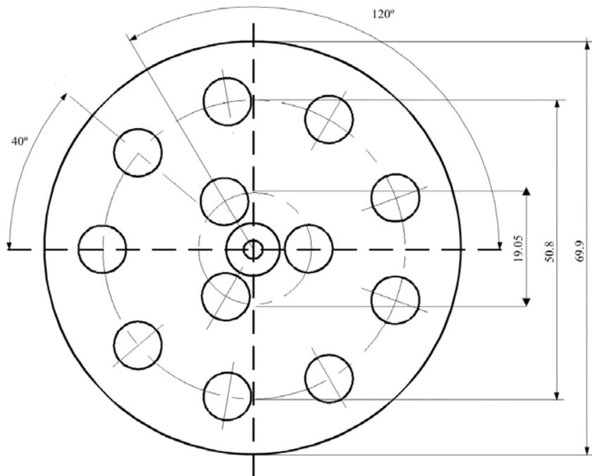
Tolerances not specified are  $\pm 0.1 \text{ mm.}$ "
