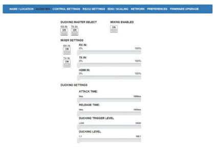
MIXING ENABLED: Click the button to set audio mixing function to ON/OFF. The default setting is OFF.
