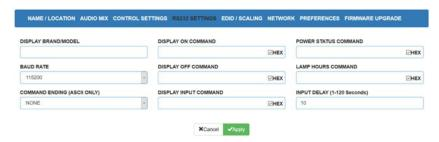
This tab allows you to define the RS232 display control commands. If a display requires hex commands, make sure the HEX box is checked.
