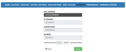
This tab allows you to select between dynamic and static IP addressing.
