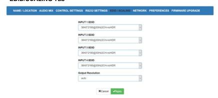
This tab allows you to configure each input EDID and the output resolution.
