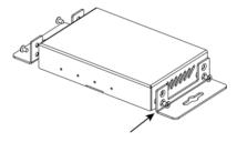
3. Attach the brackets to the surface you want to hold the unit against using the screws (provided by others).
