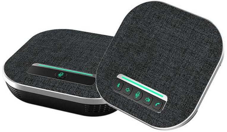
DVDO-CRSP-1 is a speakerphone kit for conference room applications that includes a main speakerphone and an extension speakerphone. The two speakerphones connect to each other over RJ45 and use 4 microphone arrays with a 360° voice pickup range up to 8m / 26ft.
