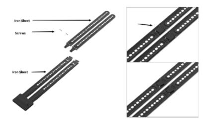
1. Join the two pieces together with the 4 SM3 screws.
