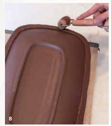
Flatten the rim down using a wooden pony roller.
