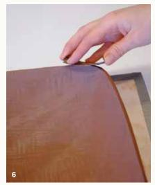
Refine the shape of the platter with a rasp, then bevel the angle of the rim inward.
