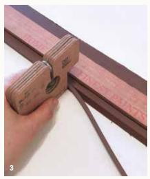
Cut a bevel with a 60° angle on a strip of clay for the foot ring.
