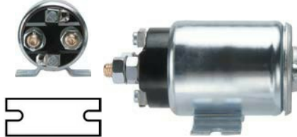
333152 Solenoid Manufacturer: Bosch replacing: 19024760 24 V, 150 a, Intermittent load 800 Amp., OD 51.50, Coil bolt M8, seconds 5, No./ terminals 4 Silver contact. Insulated return. alternative no.: 131372
