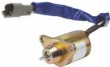
090430 Shutdown Solenoid servicing: Kubota 12 V, Plunger Internal, switch Internal This solenoid can switch off the pull coil, and no external 'control' is necessary.
