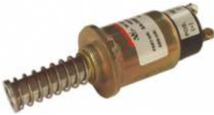
090334 Shutdown Solenoid servicing: Sisu Diesel 8366 40253 12 V, Plunger Internal, switch Internal This solenoid can switch off the pull coil, and no external 'control' is necessary.
