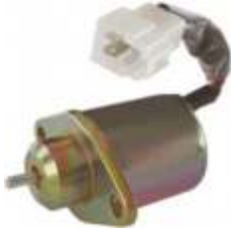
090402 Shutdown Solenoid servicing: Kubota super 5 series 24 V, Plunger Internal, switch Internal This solenoid can switch off the pull coil, and no external 'control' is necessary.
