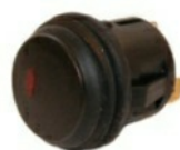
K488 Red Illuminated Push On/Off Switch With Splash Proof Seal 10A @ 12V, 12V LED Fits 20mm round hole
