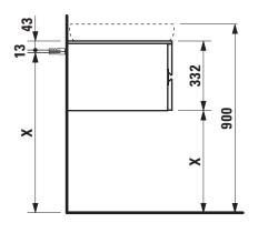
X =The exact hight must be set during installation.
