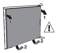
3. After removing the inner glass it is possible to access the drip catcher strip.
