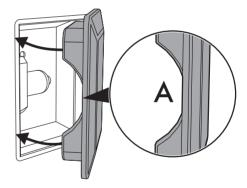
Press the cover completely down so that it attaches perfectly to the bulb support.
