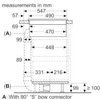
A: With 90° "S" bow connector (available from 05/2021 on) B: With 90° "L" bow connector
