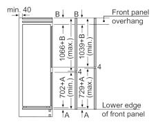
The specified unit door dimensions are valid for a door gap of 4 mm. measurements in mm Air outlet min. 200 cm<sup>2</sup> min. 560 recommended min. 550 1772<sup>+8</sup> Ventilation space in the base min. 200 cm 2 measurements in mm
