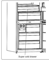
Keeping food in the super cold drawer, instead of the freezer or refrigerator compartments, allows food to retain freshness and flavour for longer, while preserving its fresh appearance. When the super cold drawer tray becomes dirty, remove it and wash with water. (Water freezes at 0°C, but food containing salt or sugar freezes at temperatures lower than this).
