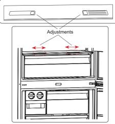
If the fruit and vegetable drawer is full, the fresh dial located in front of the drawer should be opened. This allows the air in the fruit and vegetable drawer and the humidity rate to be controlled, to increase the life of food within. The dial, located behind the shelf, must be opened if any condensation is seen on the glass shelf.
