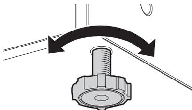
Lean the appliance slightly towards the rear part to facilitate proper door closure.
