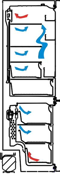
freezer and refrigerator compartments, therefore preventing the mixing of odours.
