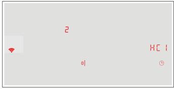
Use the "Home Connect" SSID and the "Home Connect" key to log your mobile device into the hob network.
