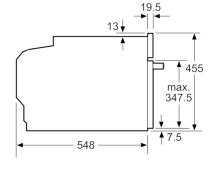
measurements in mm
