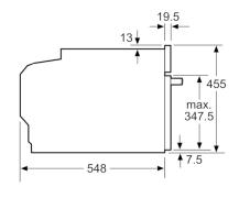
measurements in mm
