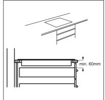
If the appliance is installed  $(\mathbf{i})$ above a drawer, the hob ventilation can warm up the items stored in the drawer during the cooking process.
