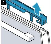
3. Lift out the inner panel (fig. 3) and set it down carefully on a flat surface.
