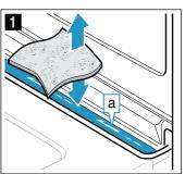
The drip trough **a** is located below the cooking compartment (figure 2).
