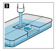
6. Insert the filled water tank (Fig. 4). Ensure that the water tank locks into place behind both holders a (Fig. 5).
