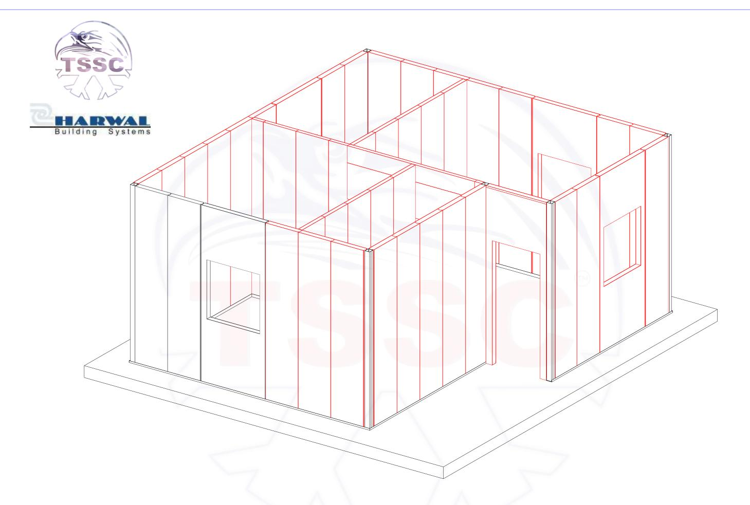
STEP 5: INSTALL ALL THE REMAINING EASYWALL PANELS AND LGS FRAMES
