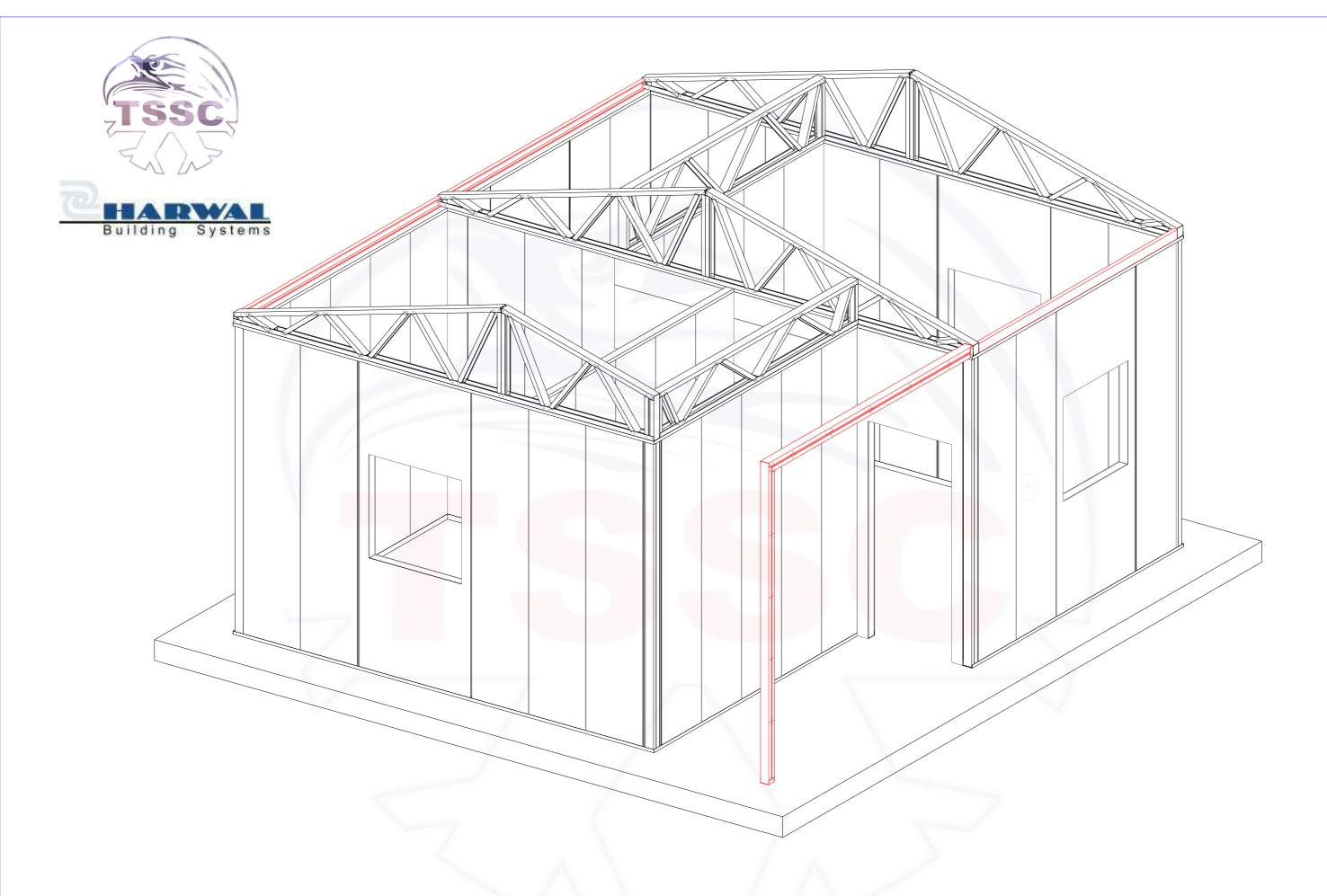
STEP 8: INSTALL THE COLUMN & BEAM AND EAVE PURLINS
