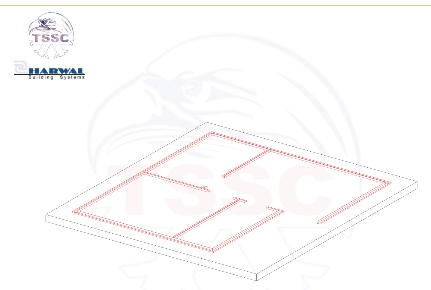
STEP 1: BASED FROM THE FLOOR PLAN DRAWING, INSTALL ALL THE BASE TRACKS (U CHANNEL) BY SCREWING TO THE CONCRETE FLOOR.
