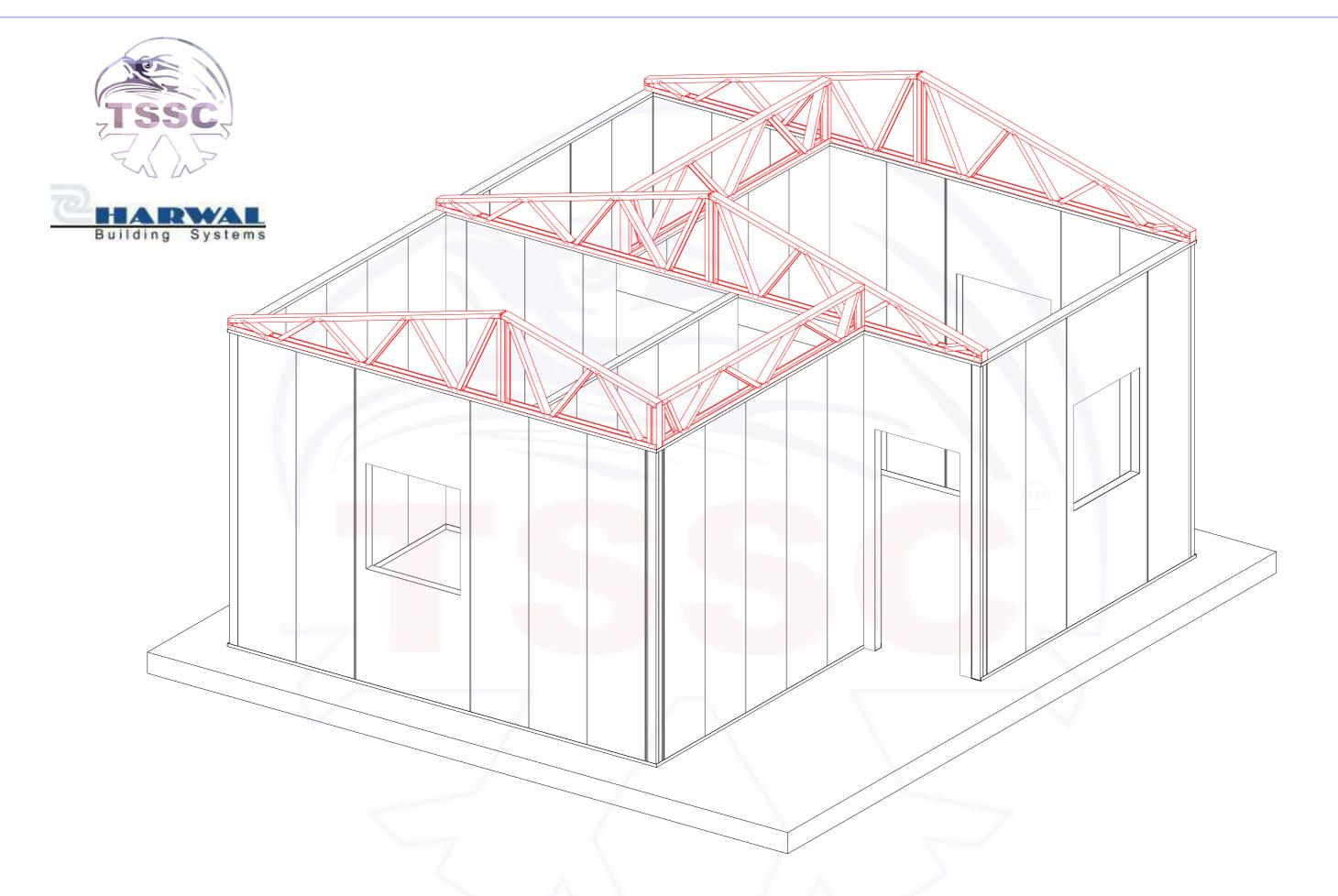
STEP 7: BASED FROM ROOF FRAMING PLAN, INSTALL THE ROOF TRUSSES
