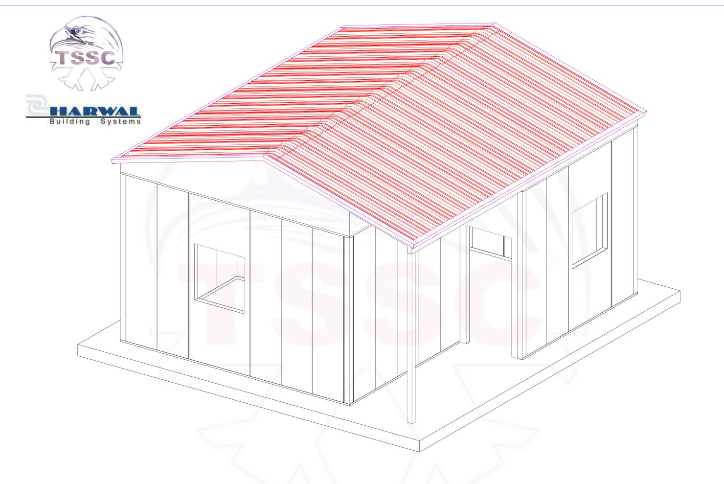
STEP 11: FIX THE ROOF SANDWICH PANELS AND FLASHINGS
