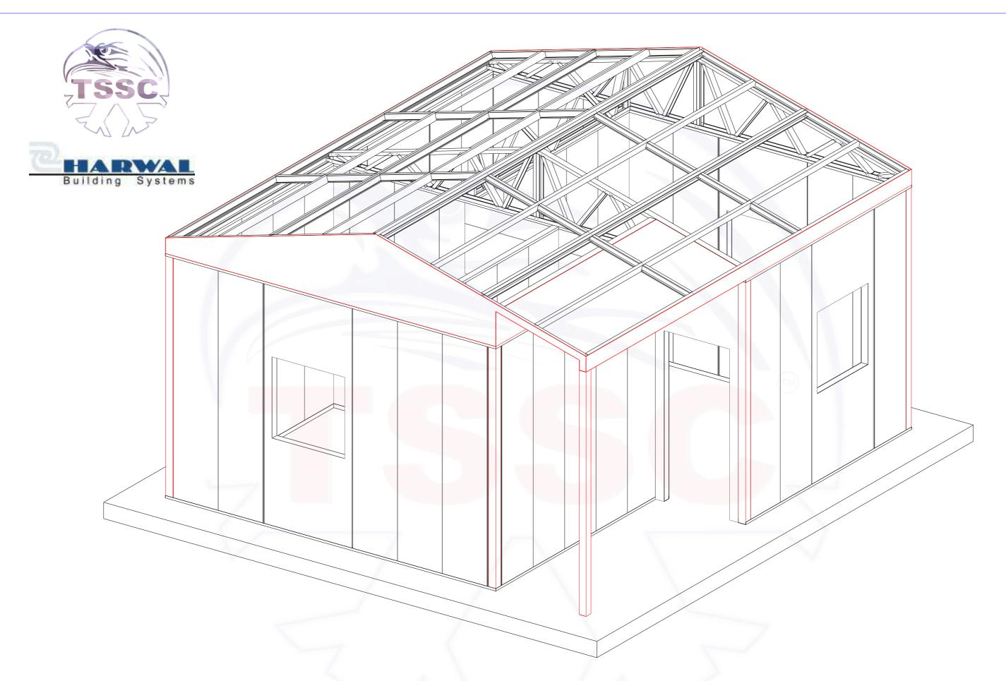
STEP 10: FIX THE CEMENT BOARD TO CORNER COLUMNS, WALL AT GABLE SIDE AND SOFFIT
