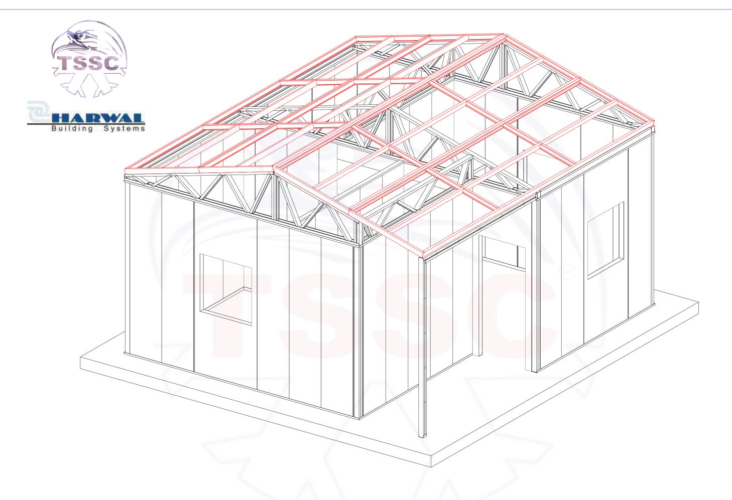
STEP 9: PLACE THE ROOF FRAME ON TOP OF ROOF TRUSSES
