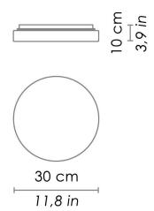
Wall-ceiling lamps with diffuser in mouth-blown, satin-finish opal triplex glass; chlorine-resistant, anti-UV, neutral translucent polycarbonate frame. Twist-lock coupling system for the glass component. The product is suitable for indoor use only. The Drum collection is IP44.
