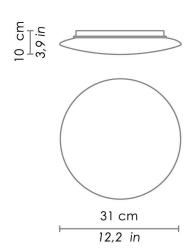
Wall/ceiling lights in satin finish triplex opal blown glass, with embossed aluminium internal reflector and a chlorine-resistant, anti-UV, neutral translucent polycarbonate base. Twist-lock system for the glass component. The Bis collection has IP44 protection.
