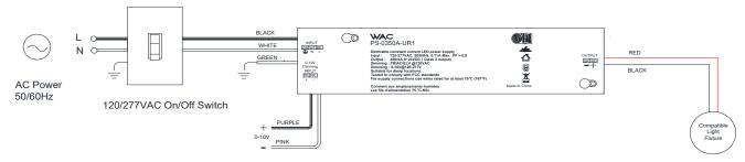
\*Note: Longer distance than 100ft between power supply to light fixture requires larger conductor wire than 18 AWG to lower voltage drop across the wire. Excessive voltage drop on conductor wires may lead to an inoperative of power supply.
