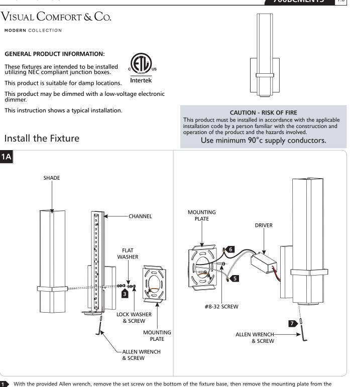
2 Install the mounting plate to the junction box with the two #8-32 screws provided.
