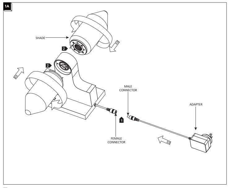
Connect the male connector from the adapter to the female adapter on the fixture.
