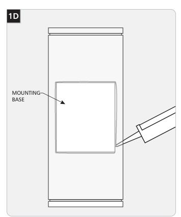
10 For wet locations, caulk around the mounting base with waterproof construction sealant.
