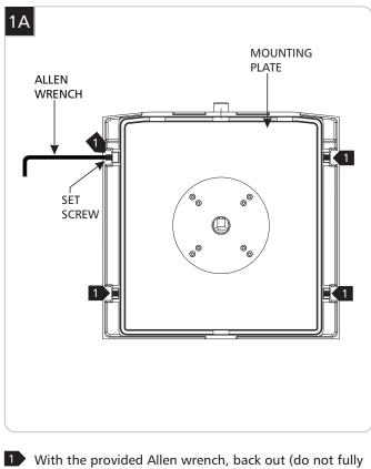
remove) the set screws on both sides of the fixture.
