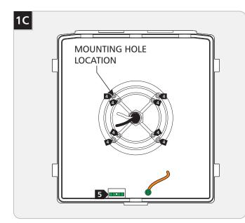
Choose and drill out the designated mounting holes that will be used to mount the mounting plate.
