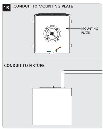
Bring conduit and power lines to the fixture location: conduit may be attached by either the center hole in mounting plate or the any of the plugs on top of the fixture. If using the top plugs, unscrew to remove.
