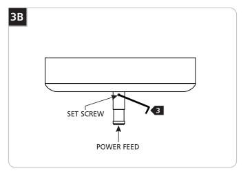
3 Loosen the set screw on the power feed.
