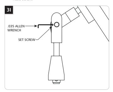
12 Tighten the set screw on the opposite side of the screw head with the provided .035 Allen wrench to ensure the position of the adapter.
