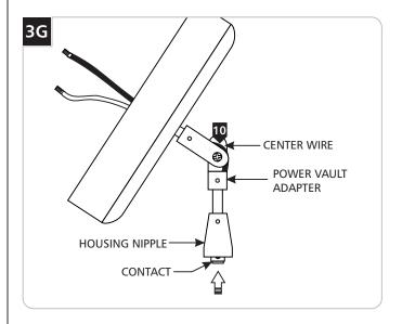
Loop the center wire and feed it completely through the second portion of the power vault adapter into the canopy.
