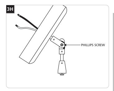
Ensure that the adapter is level and tighten the Phillips head screw.
