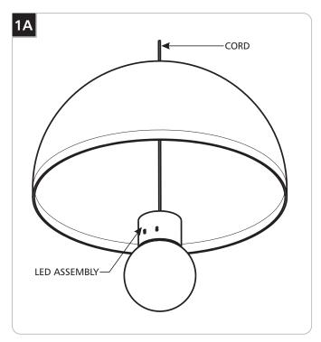
1 Feed the cord through the shade and carefully lower the shade until it rests properly on the LED assembly.
