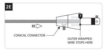
7 Feed and push the coaxial cable into the conical connector. The coaxial cable will come to a stop point after being inserted 3/4" into the conical connector.
