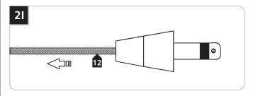
**12** Pull the coaxial cable toward the fixture to smooth the wrinkles.
