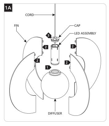
1 Carefully threaded the diffuser onto the LED assembly.
