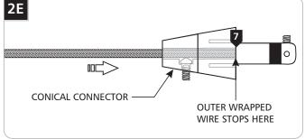
7 Feed and push the coaxial cable into the conical connector. The coaxial cable will come to a stop point after being inserted 3/4" into the conical connector.
