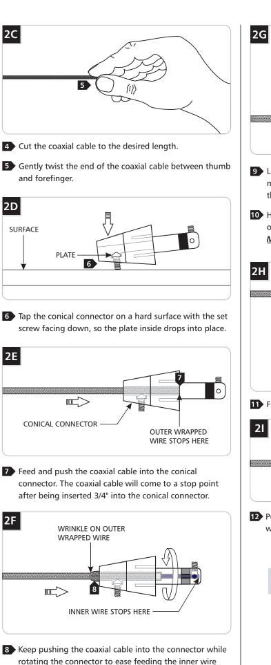
screw facing down, so the plate inside drops into place.
