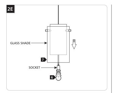
6 Push the lamp shield onto the spring clip.
