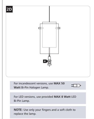
4 Gently insert the new lamp into the socket.
